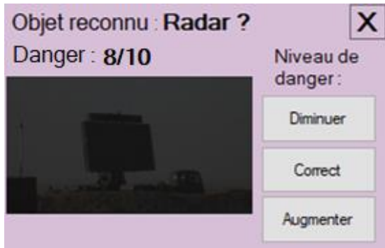
Fig. 2. Tool for checking the classification of an enemy by the operator.
